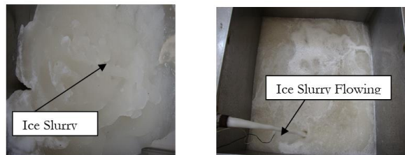
(a) Ice Slurry (b) Ice Slurry flowing in thermal storage tank
